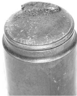
Figure 6 - Polished Rod Pin Failure
