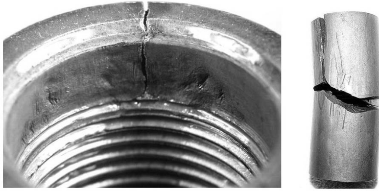
Figure 5 - Sucker Rod Coupling Failure
