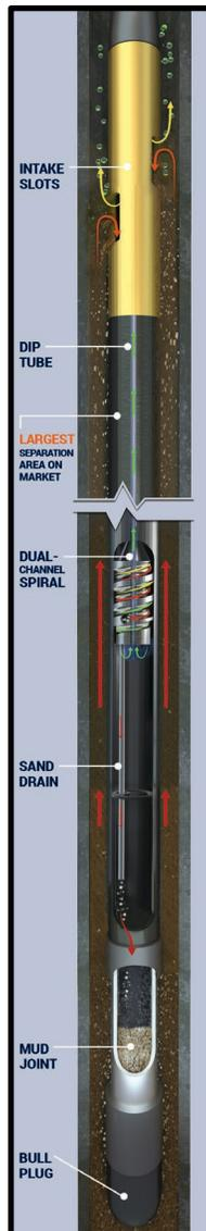
Figure 5: Schematic of the separator
