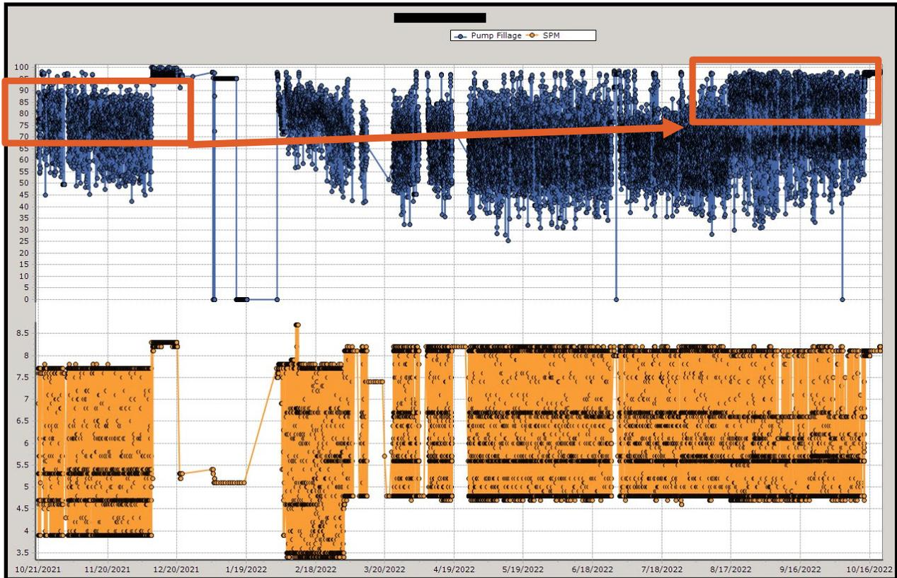
Figure 9 – Pump Fillage and SPM trend for Well 1.
