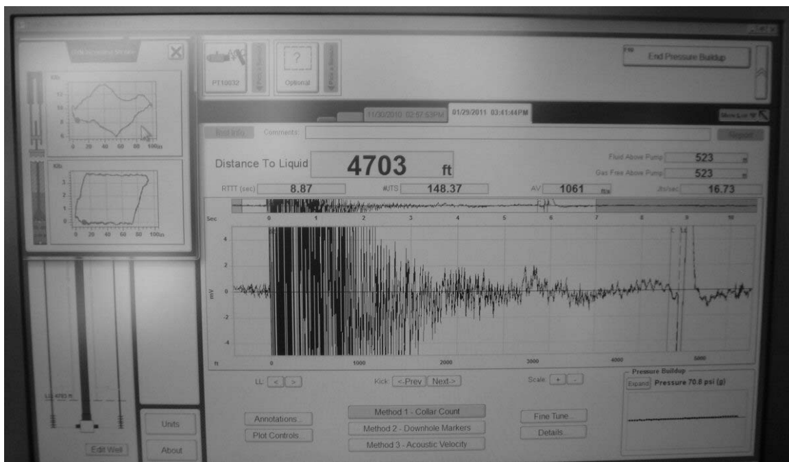
Figure 4 - Simultaneous Real-time Monitoring of Dynamometer and Acoustic Fluid Level Acquisition.
